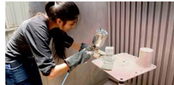
The Paint Shop is a place where students give surface treatment to their prototypes or models with the aim to give a final finish to their products. Students work with water and solvent-based paints, varnishes, various surface treatment agents, oils and waxes for this process using paint spraying booths.
