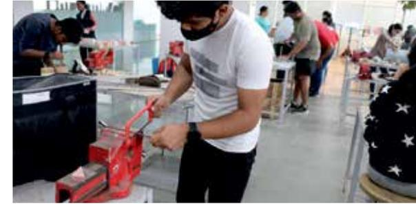
The Fitting Shop is a place where the students refine their products to achieve desired shapes, size and accuracy, through various finishing operations such as marking, filing, chipping, sawing, scraping, drilling, reaming, tapping, threading and grinding etc. The Fitting Shop includes, Machine Vice, Bench and Hand Drill Machine, Angle Grinder 540W with Angle Polisher Attachment, and various files etc.
