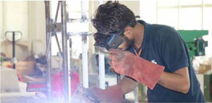
Welding Shop is a place where the students perform arc welding fusion processes for joining metals. The different operations practiced by students in Welding Shop are Position Welding, Butt Welding, Lap Welding, Spot Welding, etc. The Welding Shop includes ARC+ Tig Welding Machine with safety equipments.
