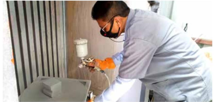
The Paint Shop is a place where students give surface treatment to their prototypes or models with the aim to give a final finish to their products. Students work with water and solvent-based paints, varnishes, various surface treatment agents, oils and waxes for this process using paint spraying booths.
