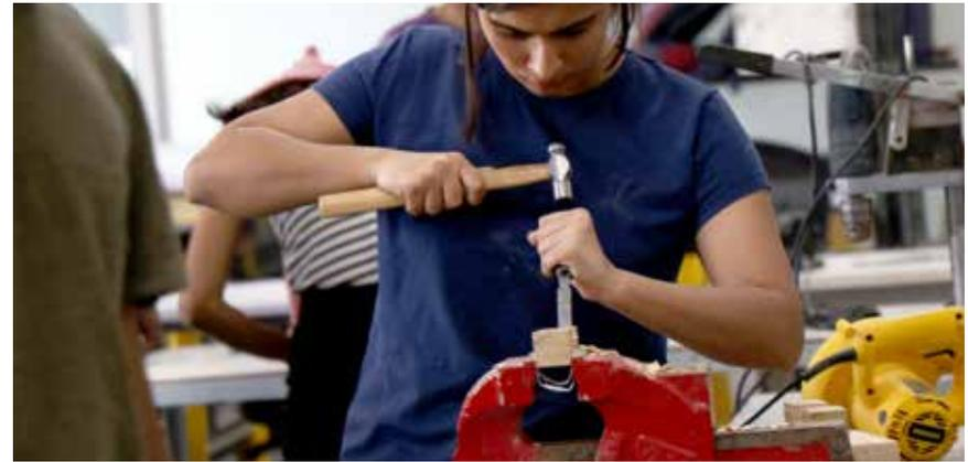
The Fitting Shop is a place where the students refine their products to achieve desired shapes, size and accuracy, through various finishing operations such as marking, filing, chipping, sawing, scraping, drilling, reaming, tapping, threading and grinding etc. The Fitting Shop includes, Machine Vice, Bench and Hand Drill Machine, Angle Grinder 540W with Angle Polisher Attachment, and various files etc.
